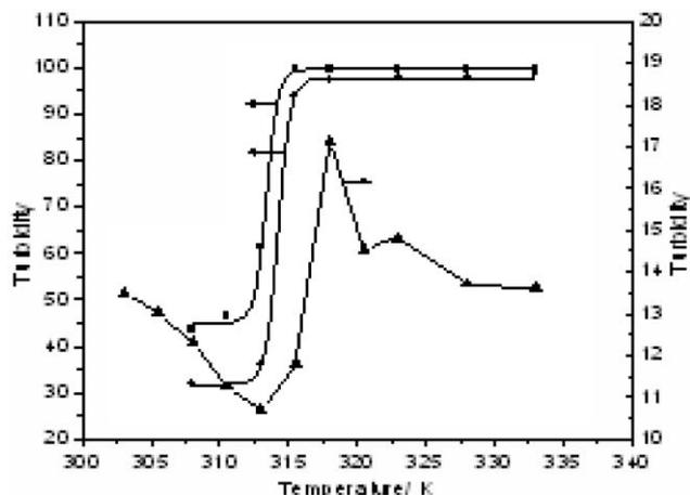
Fig. 2 Plot of turbidity of hydrogel (4 mM) versus temperature for [1] : [SDS] = 0.67 (■), 0.33 (●) and 0.25 (▲).
