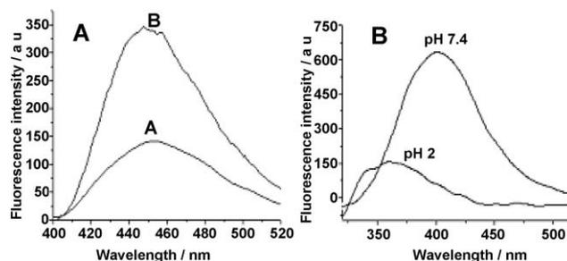
Fig. 6 (A) Fluorescence emission spectra of C-1 in gel at 25 °C, A, and in broken gel at 60 °C, B. (B) Fluorescence emission spectra of warfarin in gel (pH 2) and in broken gel (pH 7.4) measured at 30 °C.
