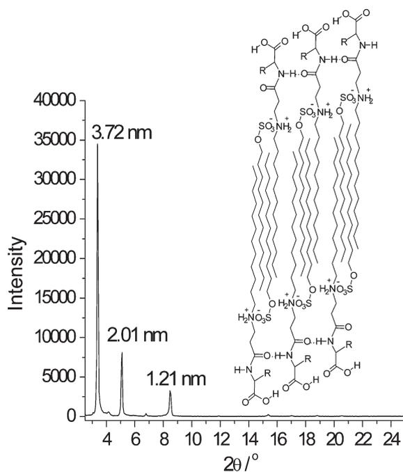
Fig. 4 X-ray diffraction pattern of hydrogel film, inset: schematic presentation showing arrangement of molecules in the bilayer self-assembly.
